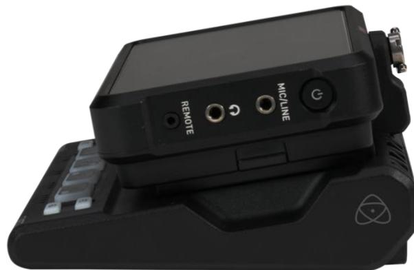
To the computer Ninja CAST appears as a high-quality webcam, so it works immediately with all video applications like Zoom, Microsoft Teams and Skype as a UVC input without a need to install drivers on the computer. There's no need to worry about synchronization, as you can mix and match frame rates as well as interlaced and progressive HD sources automatically.
