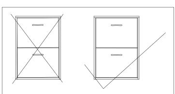
If the drawer's two side gaps were not aligned, please pull out the back panel nails and adjust the cabinet angles to ensure the frame angles are square. After the drawers are fully aligned and travel smoothly, fully hammer nails to inside back panel.
