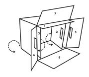
5. Rotate carton and fold out flaps 2 & 3 to form double walls
