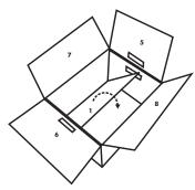
6. Tip carton on base and fold down flap 1 to form double base
