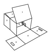
1. Break perforation to separate flaps from carton body and square up
