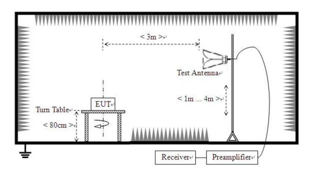
(For Radiated Emission Test (above 1 GHz))
