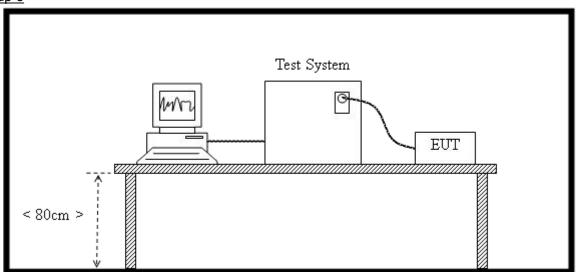
(For Harmonic Current Emissions Measurement Test)
