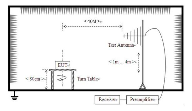
(For Radiated Emission Test (30 MHz-1 GHz))
