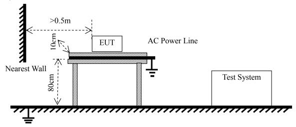
(For Electrical Fast Transient / Burst Immunity Test)
