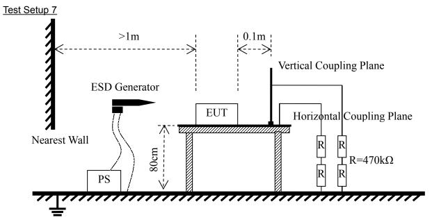
(For Electrostatic Discharge Immunity Test)
