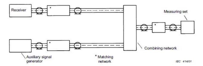
(For Conducted differential voltage emission (TV/FM broadcast receiver tuner ports))
