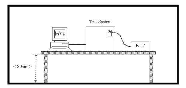
(For Voltage Fluctuations and Flicker Measurement Test)
