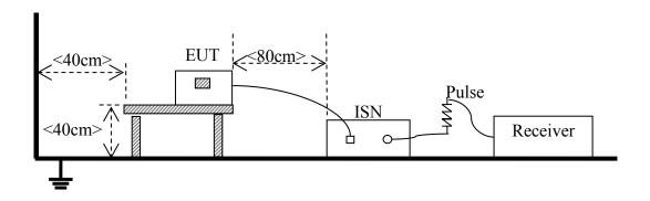
(For Conducted disturbance for asymmetric mode Test)
