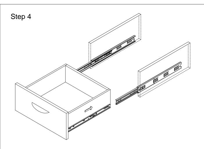
To insert drawer, fully extend both ball bearing tracks on each side and align the slide runners on the drawer with the tracks on the unit. Push the drawer into place until closed. If the drawer does not smoothly push into place, please remove and repeat insertion procedure.
