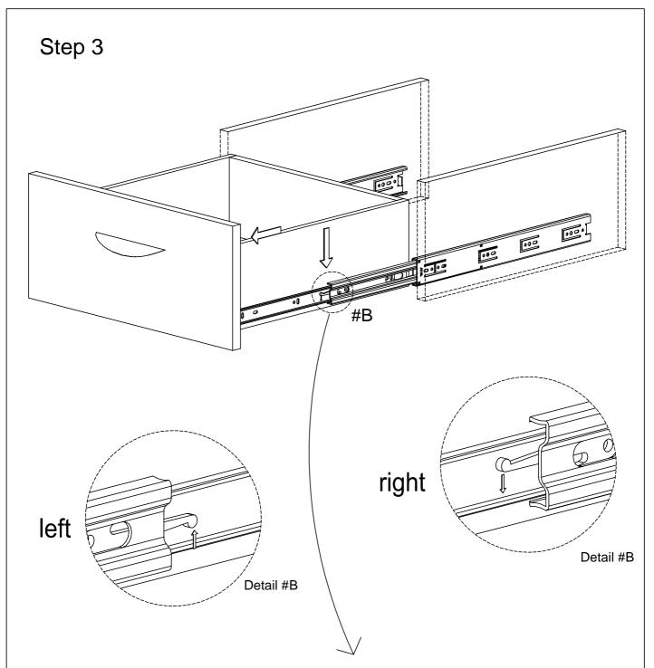
To remove drawer, pull drawer out until stopped, then simultaneously push the left plastic release lever up while pushing the right lever down, then pull the drawer out, as shown.
