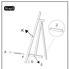
Fit part J into assembled unit as shown. Secure part K and J, using bolt A, washer and cam. Do not tighten bolt at this moment.
