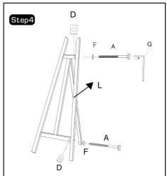
Fit part L into assembled unit as shown. Secure using bolts A, washers and cams. Now tighten all bolts using allen key.
