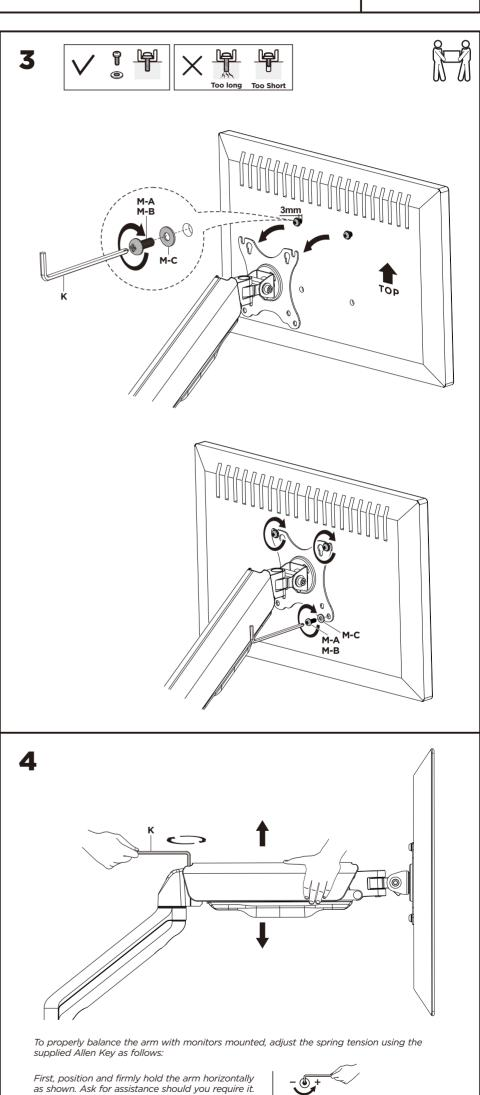
If the arm **drops**, turn the adjustment screw counter-clockwise until it stays
