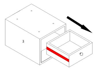
To remove drawer, pull drawer out until stopped, then simultaneously push the left plastic release lever up while pushing the right lever down, then pull the drawer out, as shown.
