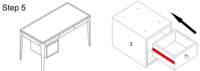
To insert drawer, fully extend both ball bearing tracks on each side and align the slide runners on the drawer with the tracks on the unit. Push the drawer into place until closed. If the drawer does not smoothly push into place, please remove and repeat insertion procedure.
