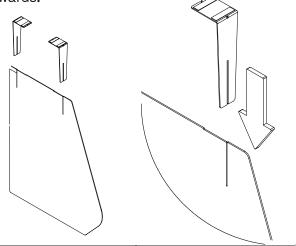
3. Test fit the screen in location without fixing it down.
