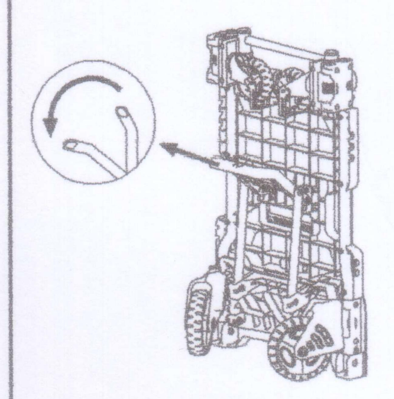
① Pull handle down to lock wheels in place.
