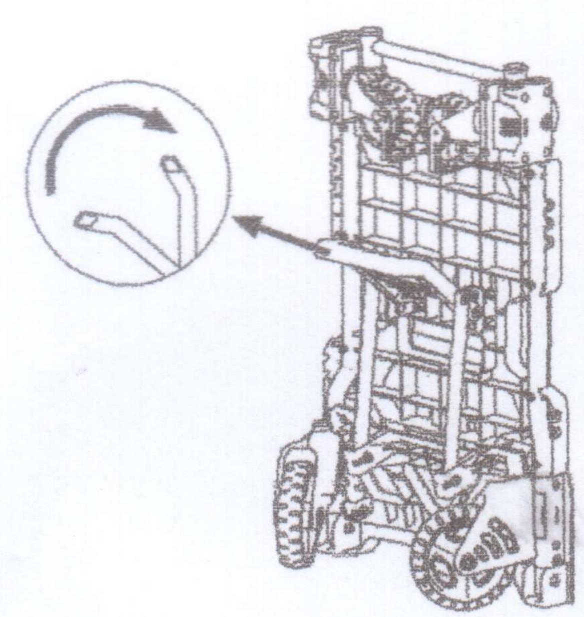
Pull handle up to retract wheels and lock in place.
