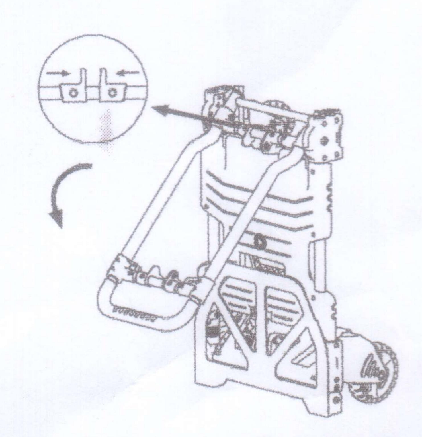
Push the handle slightly forward and backward when press the levers to unlock and fold handle down.
