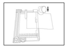
**Note:** Place the paper in the correct position as shown in images below to start cutting paper.
