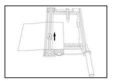
The cutting head contains a perforation blade and a wave blade. Change the blade by moving switch as per the image below.
