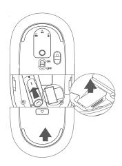
2. Place the 2\*AAA batteries(included) for keyboard and the I\*AA battery (included) for mouse into the battery compartment as per correct polarity, then take the receiver from the keyboard and close the cover.
