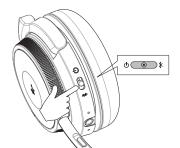
Power on: Slide the switch to the CENTRE position (Blue light illuminates for 2 seconds)
