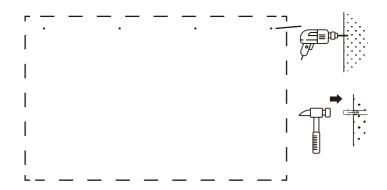
Drill 6mm diameter holes on each of the marked positions on the wall. Then hammer a Plastic anchor [B] into each hole.
