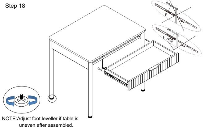
To insert drawer, fully extend both ball bearing tracks on each side and align the slide runners on the drawer with the tracks on the unit. Push the drawer into place until closed. If the drawer does not smoothly push into place, please remove and repeat insertion procedure.
