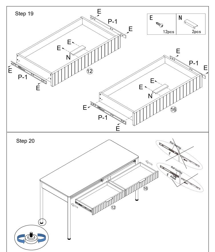
NOTE: Adjust foot leveller if table is uneven after assembled.
