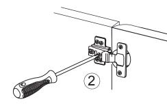
2) Depth adjustment:Loosen screw A, push hinge arm forwards or backwards, re-tighten screw A and secure screw B with a 1/4 turn clockwise.
