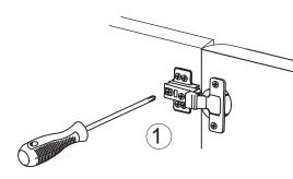
1) Side to side adjustment: Loosen screw A, adjust gap with screw B and re-tighten screw A.
