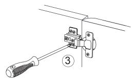
3) Height adjustment: Loosen screw C, adjust door height and re-tighten screw C.
