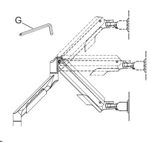
If the monitor is heavier than 4-5 kg, the arm drifts downwards.
