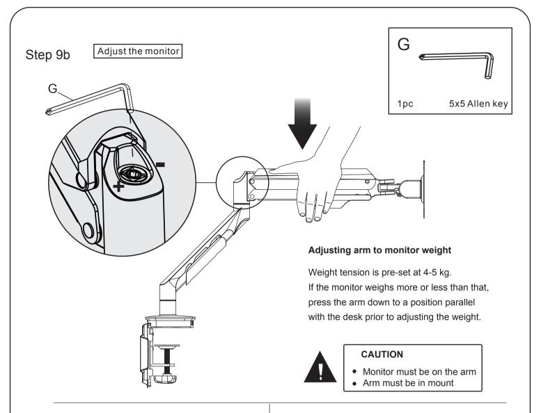
If the monitor is lighter than 4-5 kg, the arm drifts upward. Insert Allen Key (G), turn the tension screw clockwise (-).
