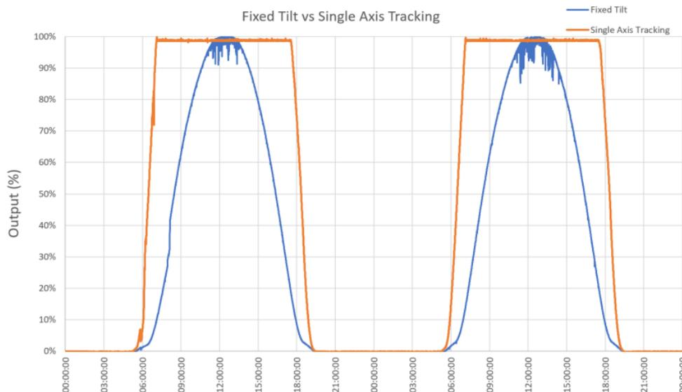
*Two days of operation on January 14 & 15<sup>th</sup> showing power output comparison. Orange line showing Northam Solar Farm data with single axis tracking, blue line showing another EMC solar farm with fixed system.*
