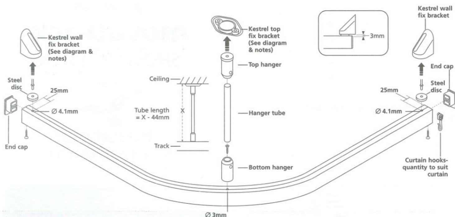
1. Check position and height of track ensuring that curtain will hang inside bath or shower tray. The aluminium track should be clear of the wall by 7mm at each end. Track may be trimmed with a hacksaw if necessary.
