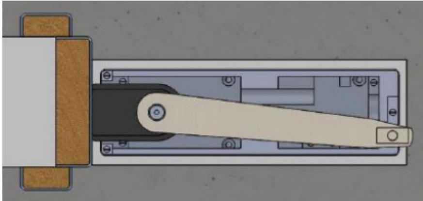
13. Open the arm to roughly  $90^\circ$  in the direction the door will open, this will require a lot of force. Lock the arm in place by carefully, slowly, tightening the  $180^\circ - 15^\circ$  screw fully clockwise. **DO NOT USE AN ELECTRIC DRIVER.**
