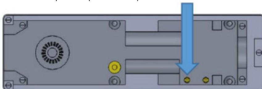
5. If the latching function is too soft to latch the door fully, begin to unscrew the latching speed screw. This should be adjusted 1/4 turn at a time. Do not fully unscrew this as the closer will be rendered inoperable permanently.
