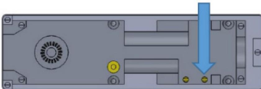
4. 1. Unscrew the closing speed screw until the door begins to close. Keep unscrewing until the desired closing speed is achieved. This should be adjusted at 1/8 turn at a time. Do not fully unscrew this as the closer will be rendered inoperable permanently.
