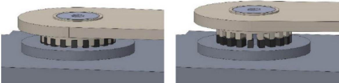
8. Lift the arm up, away from the splines and begin to open the door. As the arm rotates, push down on the arm whilst opening the door, you should feel the spline drop into the next position on the spline. The angle between positions on the spline is 18°.
