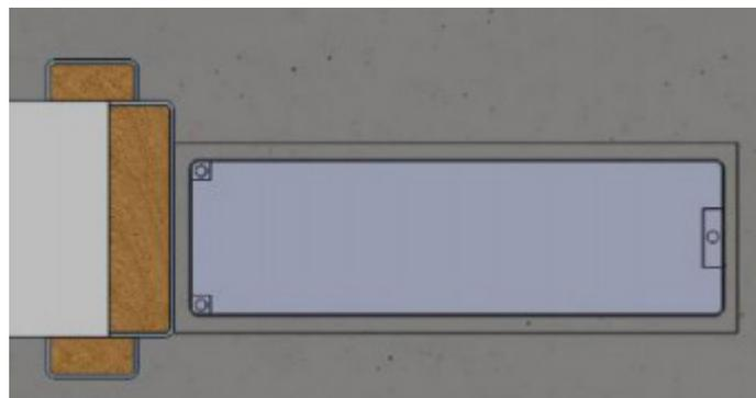
8. Once the housing is located properly, fill the surrounding area with quick drying concrete.
