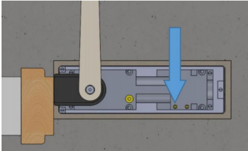
14. Mark the location of the closer arm on the closer body then remove the closer arm. This mark is needed later when the arm is re-fitted.
