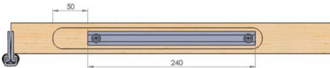
3. Install the hinge to the door. Do not hang the door.
