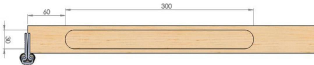
2. Leaving at least 50mm to the hinge side, fit the 240mm sliding arm channel in the rebate, using [2X] No. 10 CSK x ¼" woodscrews [Not provided]. This must be secure.
