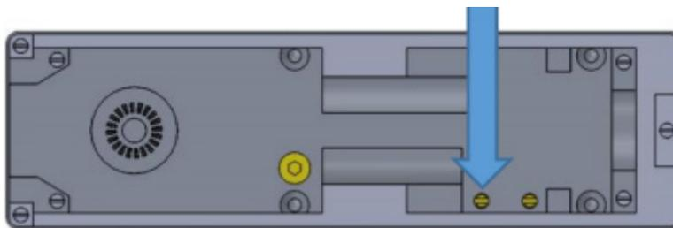
5. If the latching function is too soft to latch the door fully, begin to unscrew the latching speed screw. This should be adjusted at 1/4 turn at a time. Do not fully unscrew this as the closer will be rendered inoperable permanently.
