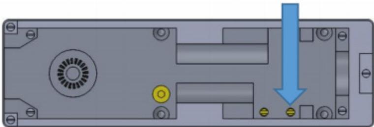
4. Unscrew the closing speed screw until the door begins to close. Keep unscrewing until the desired closing speed is achieved. This should be adjusted at 1/8 turn at a time. Do not fully unscrew this as the closer will be rendered inoperable permanently.
