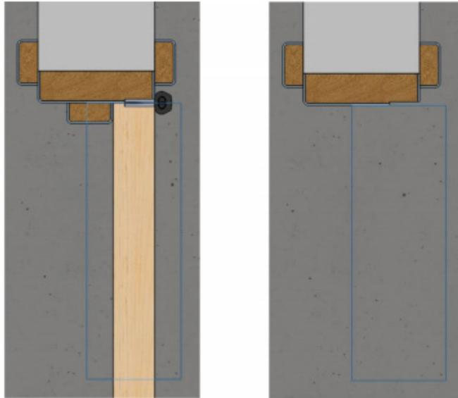
6. Remove the closer from the housing by unscrewing the 3 locking screws. Once they are loose, the closer should slide out.
