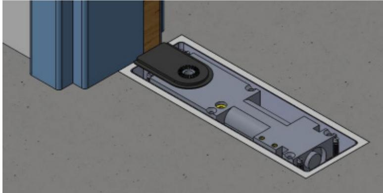
10. Use the 4 adjustment screws to fine tune the closer position, making sure the main body is flush with the floor.
