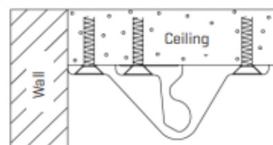
1. Correct placement facing the wall.
