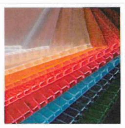
Twinwall Polypropylene Sheet is usually cut using conventional paper guillotining equipment. The material ca also be die cut or scored into a variety of shapes using standard steel rule die cutting equipment. For smaller job runs or craftwork a sharp utility knife is also suitable.
