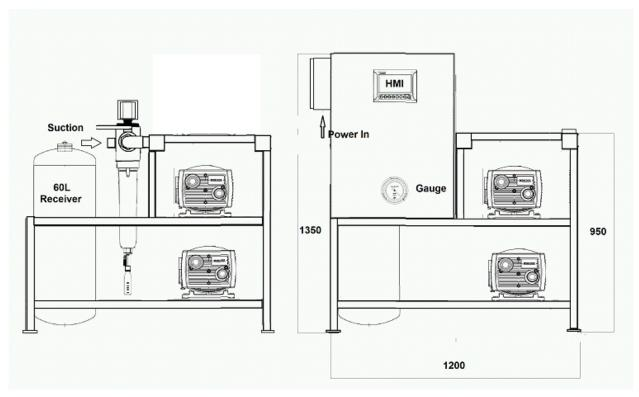
Model MS13-2-60 expandable/modular duplex central vacuum system consisting of two Becker or approved equivalent VT4.40 vacuum pumps mounted on a common skid with expandable automatic alternating electrical controls and 60Liter vertical receiver.
