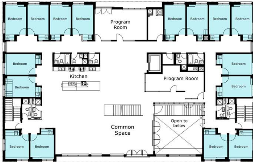
Floor plan showing 16 bedrooms gathered around a common area including a shared kitchen - 7350sf.
