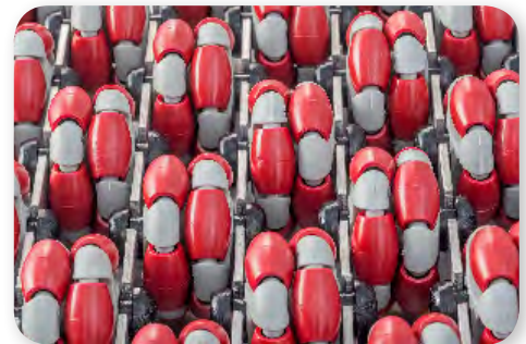
More wheels per m 2 enables greater load distribution and the ability to handle a wide range of surface profiles.
