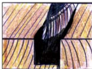
3. Apply Fixseal Epoxy Sealer
