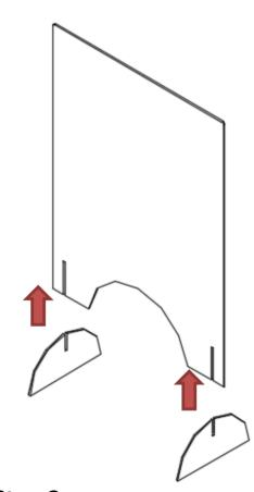
**Step 2**Slide slotted half moon bases into main screen slots and unsure fully engaged
