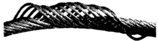
High Stranding (Only on non-rotating crane winch ropes)
