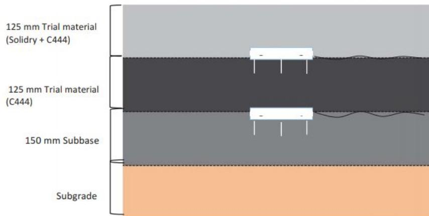
Figure 3.11 - Position of Moisture sensors in material
