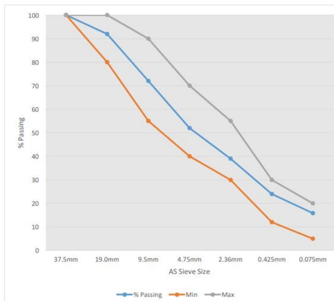
Figure 1 Recommended Grading Curves for Optimum performance with Consolid 444 and Solidry
