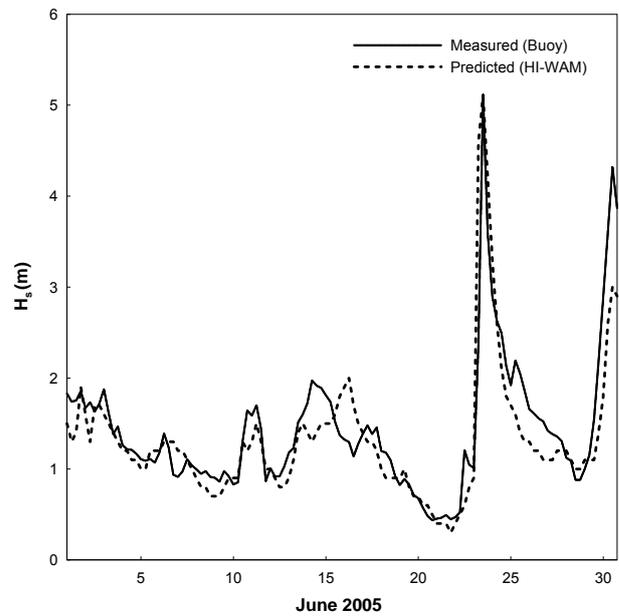
Figure 3 Comparison of the measured and predicted wave heights ( $H_S$ ) at Batemans Bay.
