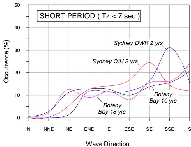
Figure 4 Wave Direction Distributions -  $T_z$  less than 7s
