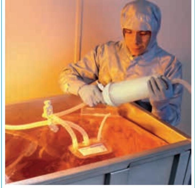
throughput performance, and assurance of process safety. Pall microbially-rated capsule filters can be supplied pre-sterilized for easy integration into Allegro™ single-use systems.
