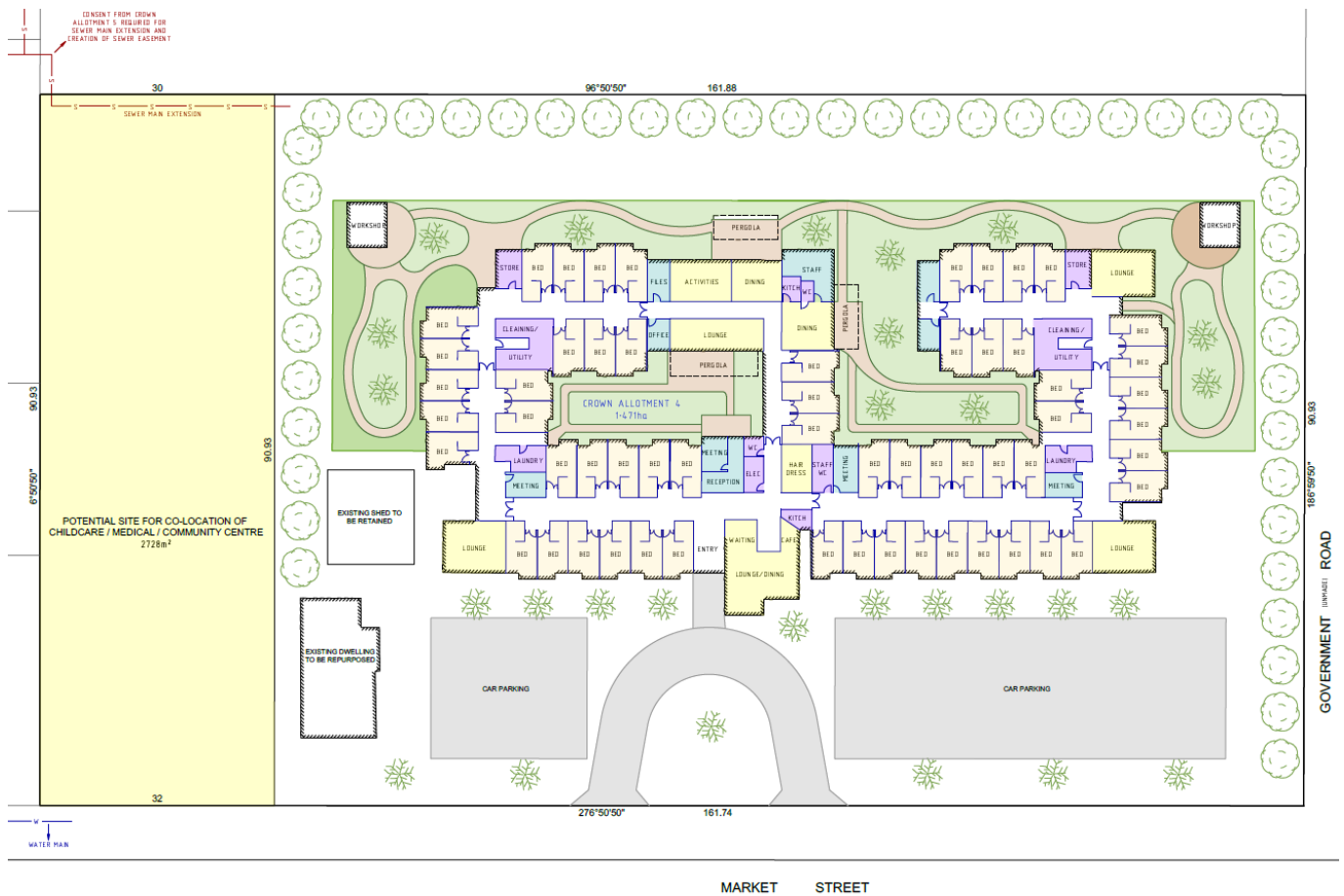
Figure 10: Indicative 58 Bed Residential Aged Care Facility Layout Plan on Crown Allotment 4. Image Source: Beveridge Williams
