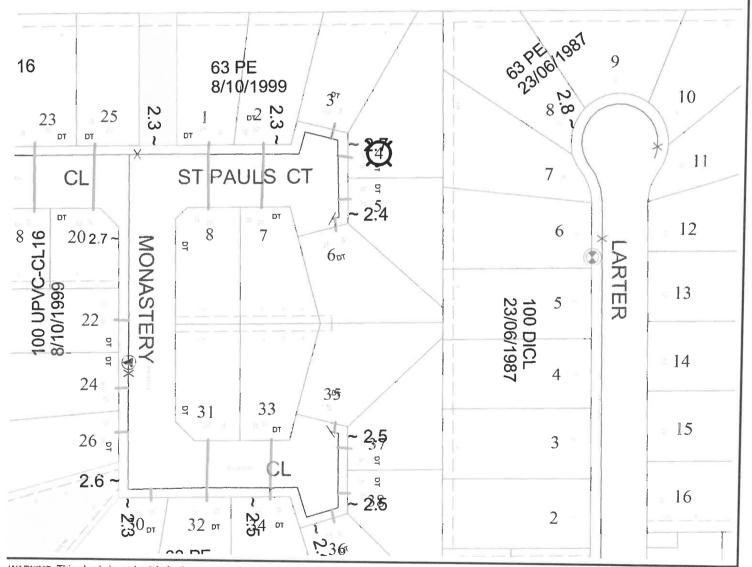
WARNING: This plan is issued solely for the purpose of assisting you in identifying South East Water's and Melbourne Water's specified assets through further investigation only. It is not to be used for any other purpose, including to identify any other assets, property boundaries or dimensions. Accordingly, the location of all assets should be proven by hand on site prior to the commencement of any work. (Refer to attached letter for further details). Assets labelled AC may contain
