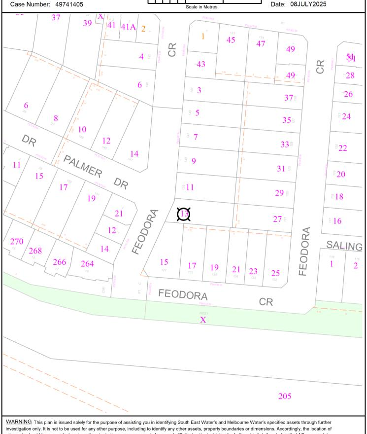
all assets should be proven by hand on site prior to the commencement of any work. (Refer to attached letter for further details). Assets labelled AC may contain asbestos and therefore works on these assets must be undertaken in accordance with OH&S Regulations. Abandoned and currently unused assets are shown in orange.
