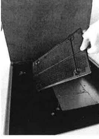
Figure 4: Air filter being removed from hatch
