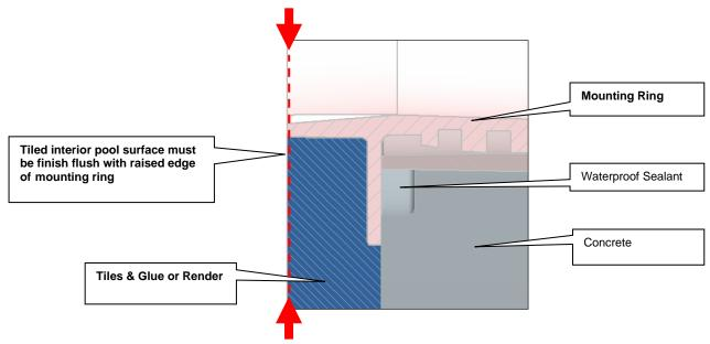
ATTENTION: Interior pool surface must finish flush with the raised edge of the mounting ring, or it will not be possible to properly install the light.
